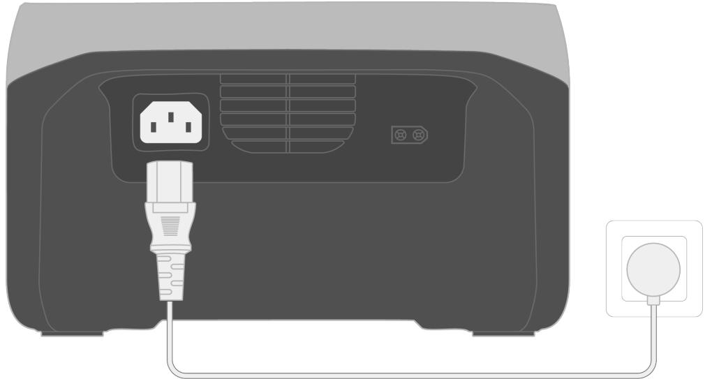
Please use the **AC charging cable** included in the package and plug the cable directly into a wall outlet instead of an extension socket.
