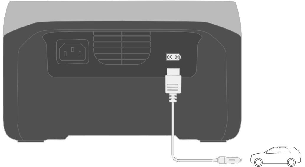
You can recharge the product through the car power outlet. The product supports 12V/24V car chargers and a maximum charging current of 8A. EcoFlow takes no responsibility for any loss or damage caused by failure to follow instructions.
