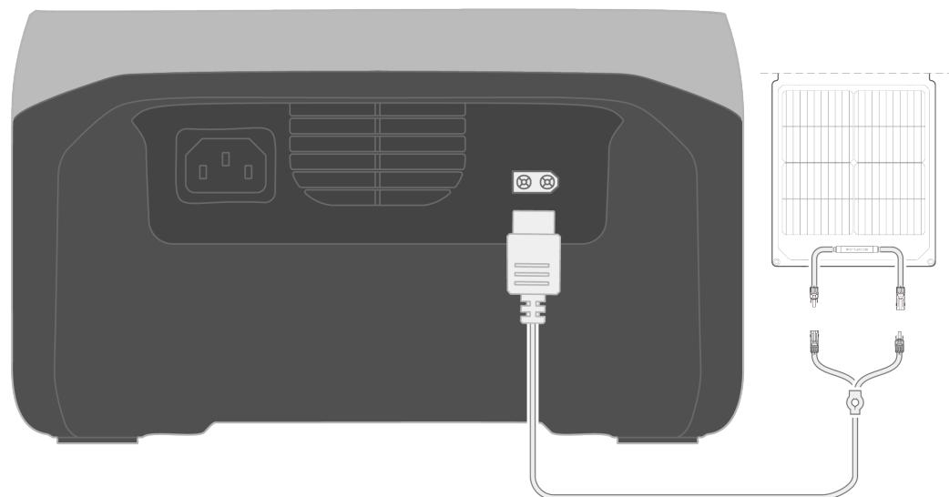
When using an [EcoFlow solar panel](#) to charge the product, connect them according to the instructions in the user manual.
