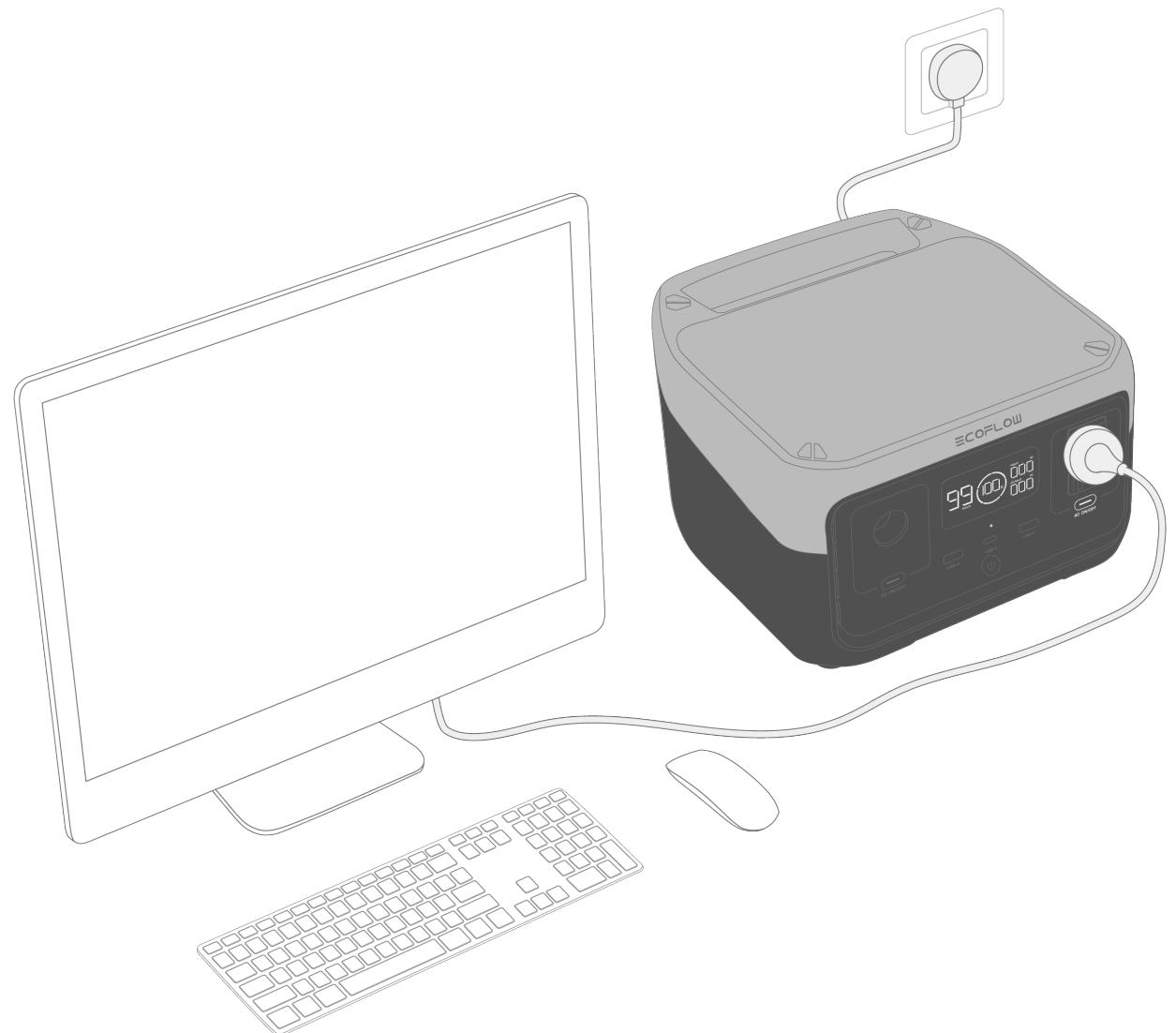
AC power will come from the grid instead of the power station in this situation (bypass mode). In case of a sudden blackout, the product can automatically switch to battery-powered supply mode within 30ms.
