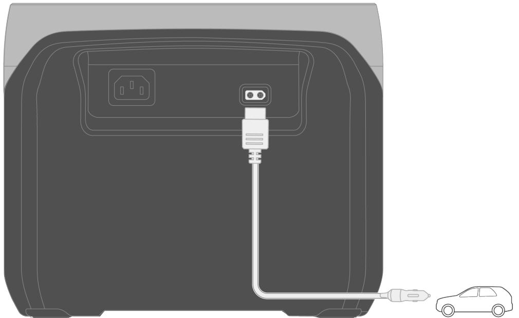
You can recharge the product through the car power outlet. The product supports 12V/24V car chargers and a maximum charging current of 8A. EcoFlow takes no responsibility for any loss or damage caused by failure to follow instructions.
