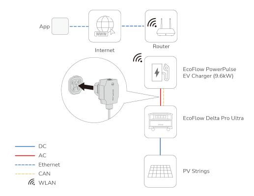
When used with DPU alone, the charger can access stored power from the battery system. This setup allows you to charge your EV even during power outages. DPU also supports integration with solar panels, offering a flexible and sustainable power solution for EV charging.
