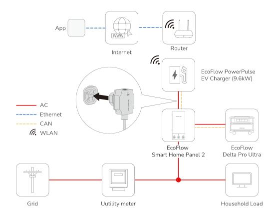
The most comprehensive setup includes both SHP2 and DPU. This combination enables full-spectrum smart energy management, with real-time control over when and how to use grid, solar, or battery power. Within this setup, you can schedule charging tasks, control power source priorities, and maintain backup readiness — all within one connected system.
