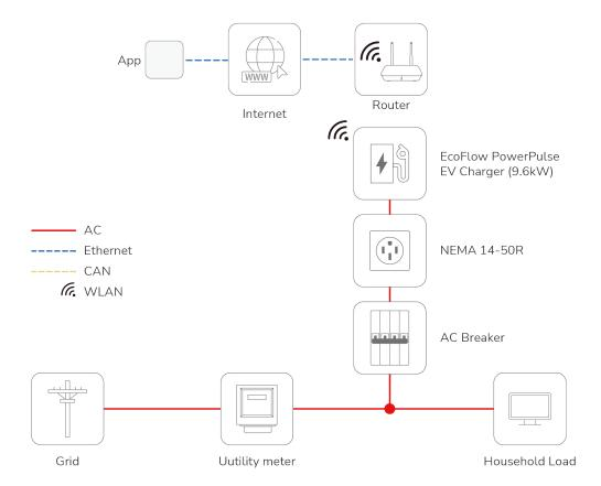
When connected solely to the grid, the charger can deliver a maximum output of 9.6 kW. In this setup, a EcoFlow Power Input Cable (NEMA 14-50P) is required for proper connection and safe operation.
